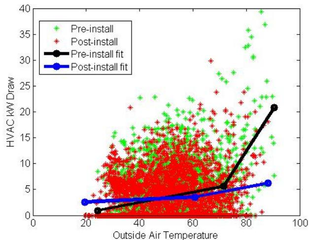
Figure 2. HVAC kW draw versus air temperature at school (October to February, 2012/13 and 2013/14).
