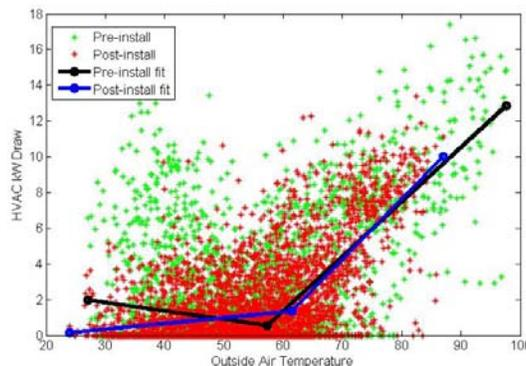
Figure 3. HVAC kW draw versus air temperature at restaurant (September to February, 2012/13 and 2013/14).
