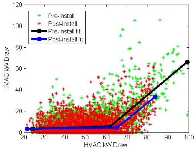
Figure 4. HVAC kW draw versus air temperature at clubhouse (September to February, 2012/13 and 2013/14).
