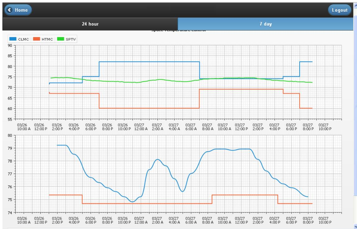
The Mobile Dashboard™ also shows the lighting schedules and the lighting operation. Technicians can proactively resolve excessive lighting runtime problems as well as HVAC and zone performance problems while at a site.
